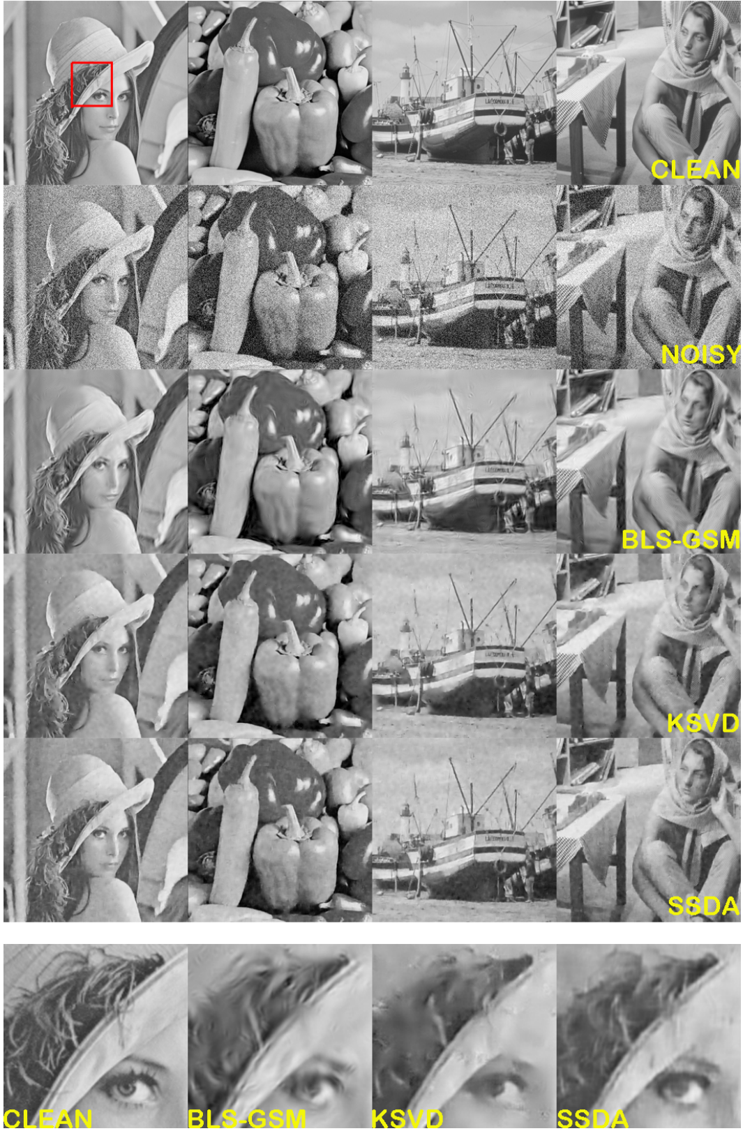
Figure 2: Visual comparison of denoising results. Results of images corrupted by white Gaussian noise with standard deviation \sigma = 50 are shown. The last row zooms in on the outlined region of the original image.
