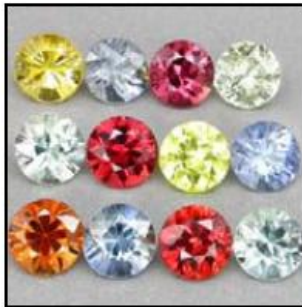
Sapphire: \text{Al}_2\text{O}_3 single crystal (corundum)! Rubine: \text{Al}_2\text{O}_3 single crystal doped with Cr!
