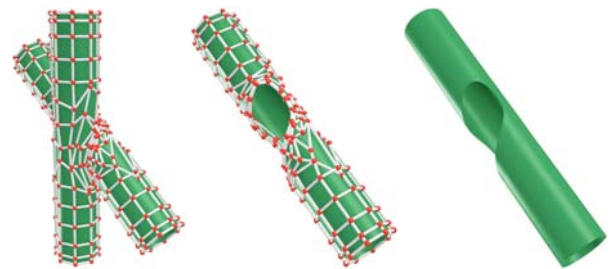
Figure 15: Trimless T-Spline Cylinders. Relative Error = 0.0009
