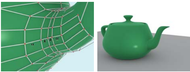
(a) Knot intervals following merge. (b) Setting k = 0.1 to create a small fillet. Initially, k = 0 .
