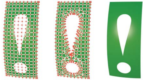
(a) Trimmed NURBS. (b) Untrimmed T-Spline. (c) Untrimmed T-Spline. Figure 7: Trimmed NURBS to Untrimmed T-Spline Conversion.
