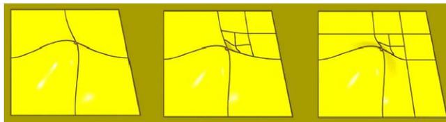
**Fig. 3** The modification of one basis function with general edge insertion operator
