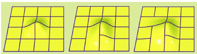
**Fig. 4** The modification of one basis functions with general edge removal operator
