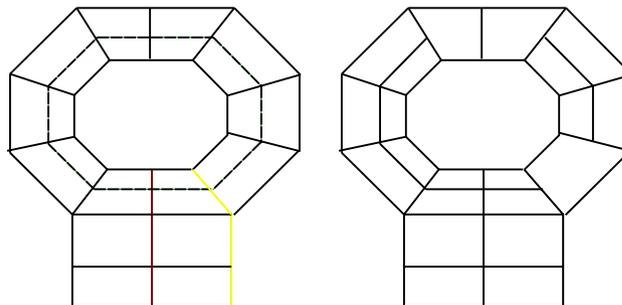
**Fig. 11** The poly-edge for a mesh. The yellow, red and the dashed lines are all poly-edges for the mesh, and the right picture is a possible removal result for the dashed poly-edge
