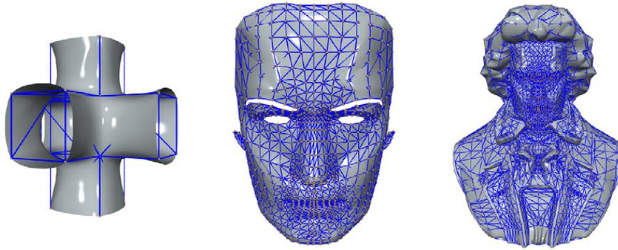
Fig. 14. Examples of applying the proposed interpolatory subdivision from Loop scheme to triangular meshes with boundaries.
