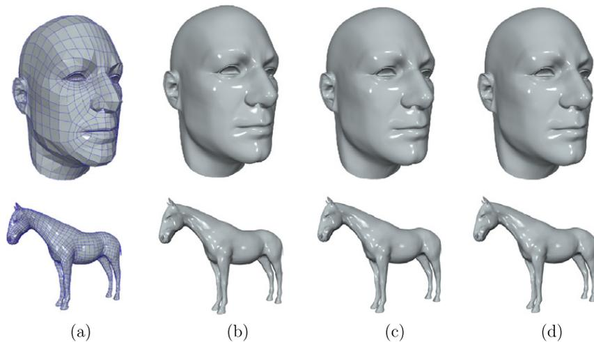
**Fig. 6.** (a) The origin meshes. (b) The results using the scheme in Kobbelt (1996). (c) The results using scheme in Lin et al. (2008). (d) The results using the proposed scheme.
