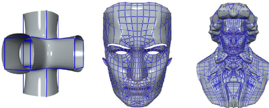
Fig. 13. Examples of applying the proposed interpolatory subdivision from Catmull-Clark scheme to meshes with boundaries.
