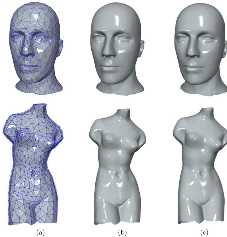
Fig. 10. (a) The initial control grids. (b) The results of the modified butterfly schemes (Zorin et al., 1996). (c) The results of the proposed scheme.
