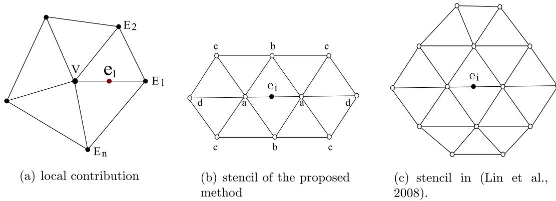
Fig. 9. The notations for the new interpolatory scheme based on Loop subdivision scheme.
