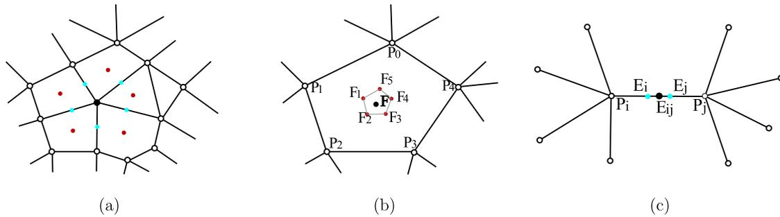
Fig. 3. Processes of the new interpolatory scheme. (a) Compute the contribution of each vertex to the neighboring face points and edge points. (b) Compute the face point as the average of the face contributions from the vertices of the face. (c) Compute the edge point as the average of the contributions from the two end vertices of the edge.
