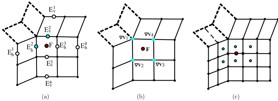
Fig. 4. Kobbelt rules (Kobbelt, 1996) and Lin et al.'s rules (Lin et al., 2008). The right figure shows the support for computing an edge point in red. (For interpretation of colors in this figure, the reader is referred to the web version of this article.)
