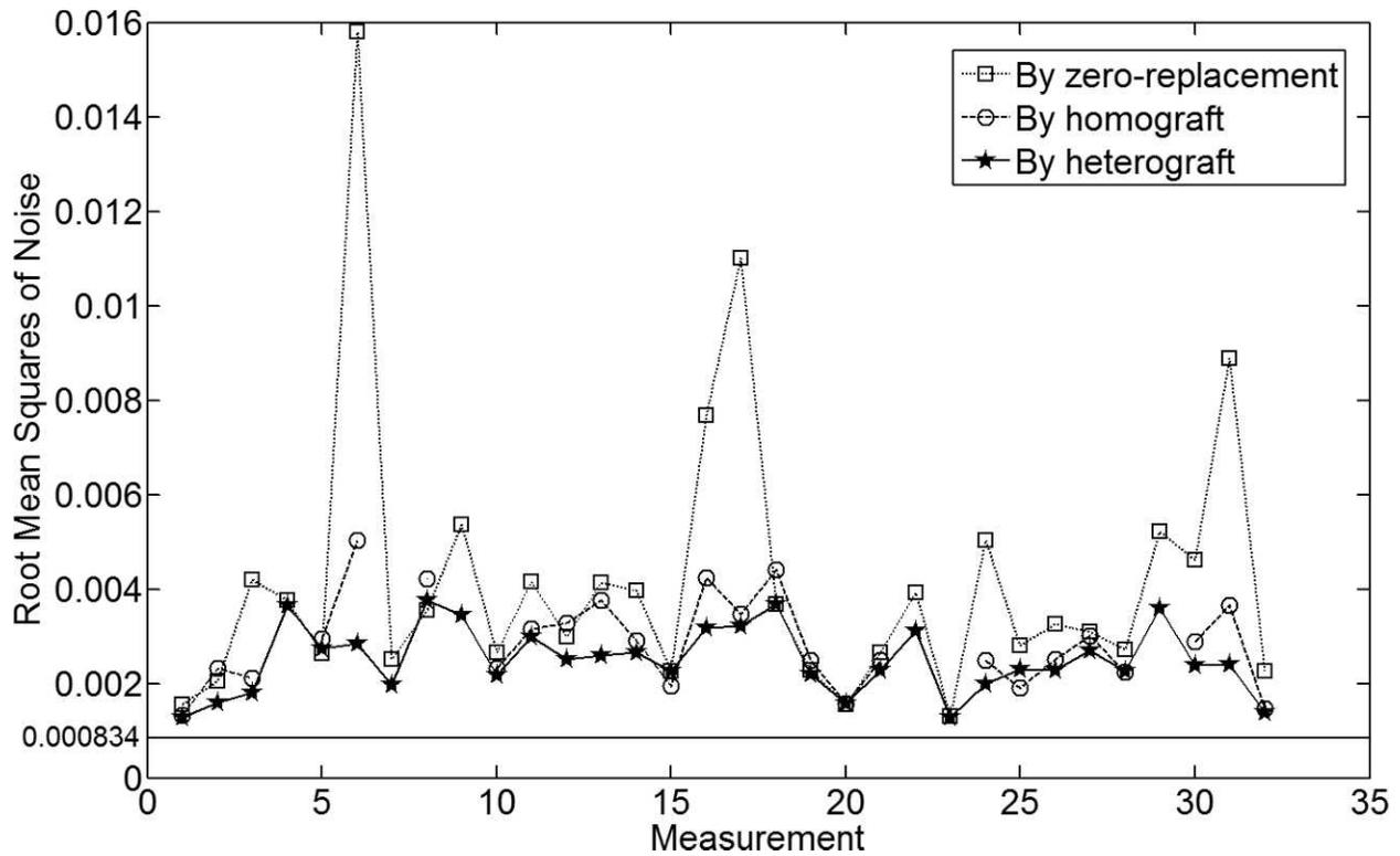
FIG. 4. The RMS noise levels of spectra computed from interferograms processed with three spike-removal techniques. The horizontal line represents the benchmark noise level, which is  $8.34 \times 10^{-4}$  a.u.
