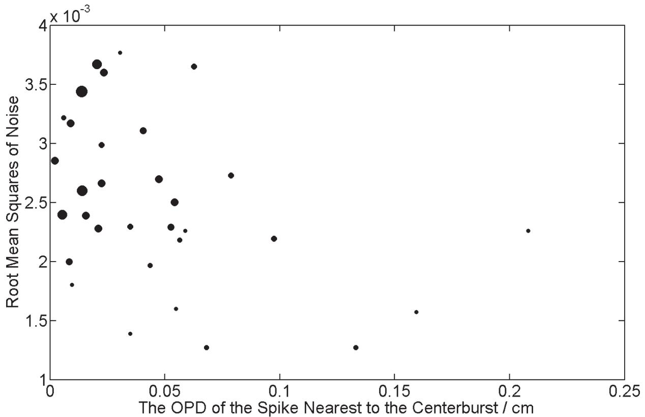
FIG. 5. The RMS noise levels of spectra from the interferograms processed with the heterograft technique. Each dot represents one interferogram, and the size is proportional to the number of spikes removed.
