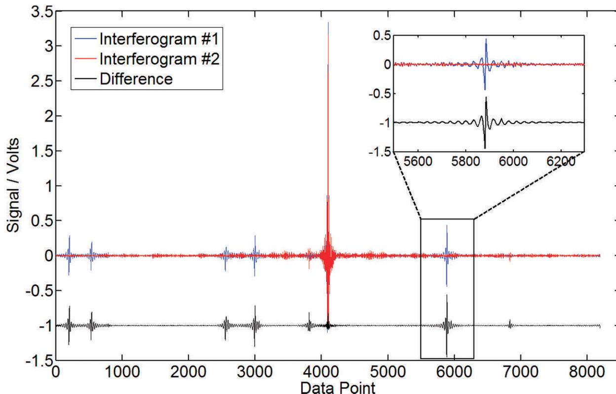
FIG. 1. Two interferograms measured consecutively in the presence of fireworks, and the difference, which is displaced for clarity. The inset shows an enlargement of one spike. The two interferograms were processed with high-pass filtering as described in the paper.
