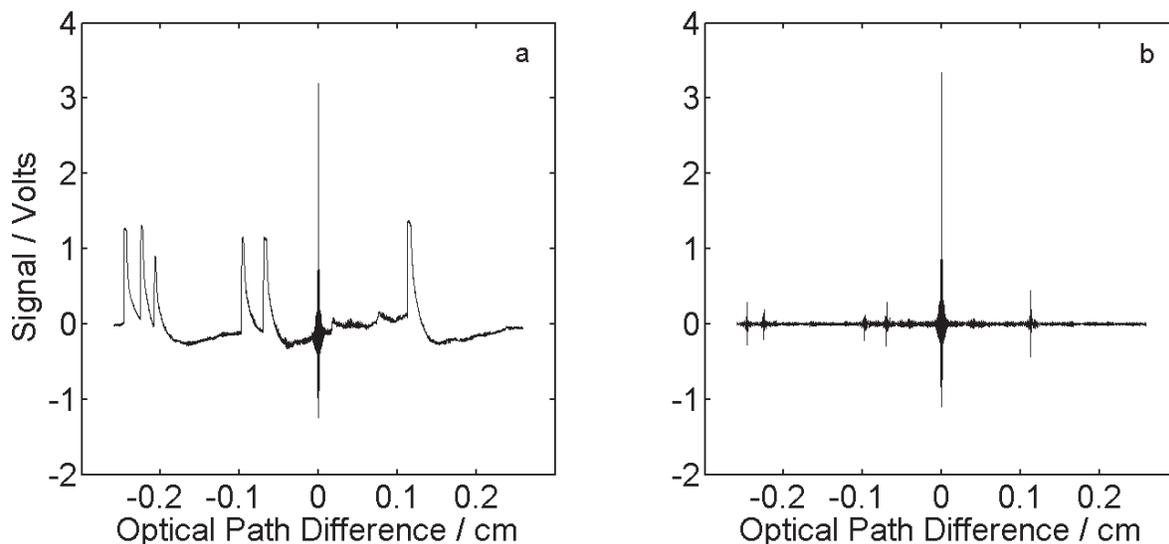
Fig. 2. A measured interferogram with extraneous sharp spikes (a) before and (b) after high-pass filtering.
