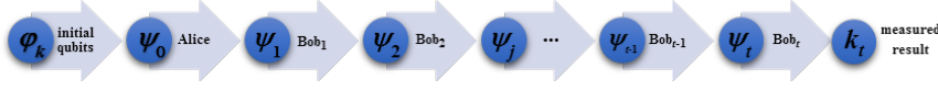
Fig. 1: Sequential operations on each qubit in Classical Information Sharing ( \varphi_k -initial phase value of each qubit |\Phi_k\rangle , k = 0, 1, 2, \dots, m ; U(\psi_0) -phase shifted by the dealer Alice on the qubit; \psi_j = (\phi_j + 2\pi c_j/p) -phase shifted by Bob_j on the qubit, j = 1, 2, \dots, t ; k_t -result measured by the last participant Bob_t .)
