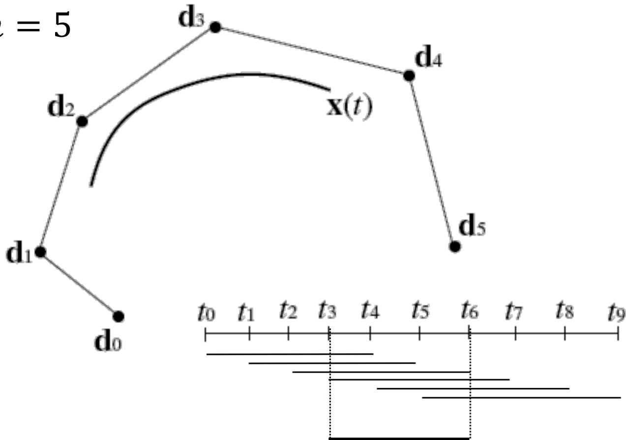
Curve defined in interval  $t_3 \leq t \leq t_6$
