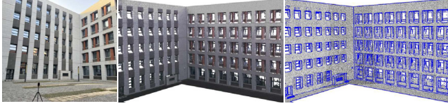
Fig. 19. Result for a LiDAR scan of a building. From left to right, the images display a photograph of the building, the raw scan, and the extraction result. Our method successfully identifies the scene structures and boundary points while excluding most false features introduced by the scanning process.
