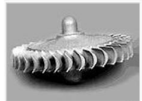
Si 3 N 4 axial rotor for a gas turbine engine.
