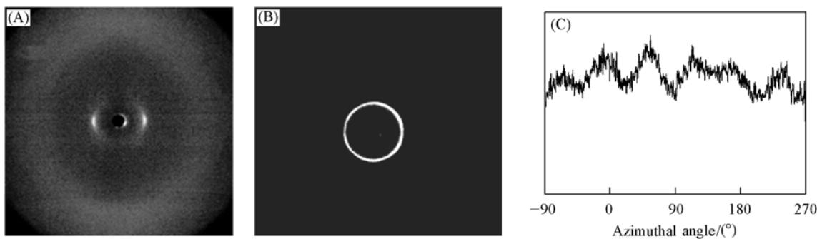
**Fig. 3** 2D WAXD fiber patterns of B-Poly-1 at room temperature
