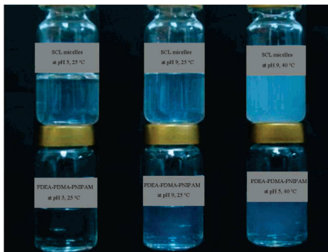
Figure 3. Digital photographs obtained for 5.0 g/L aqueous solutions of PDEA- b -PDMA- b -PNIPAM and SCL micelles at different pH's and temperatures.
