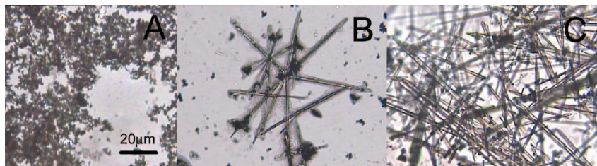
Figure 1. Morphology of the hydrothermal products at 165 °C for different times of (A) 20, (B) 30, and (C) 40 h. The bar is 20 \mu\text{m} for A–C. The molar ratio of repeating unit of HPG to \text{AgNO}_3 was 4.2:1 for all these syntheses. The images shown in A–C were taken from the as-synthesized samples, and no centrifugation was involved.
