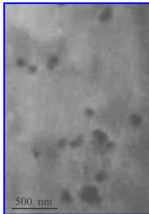
Figure 3. TEM image obtained for 10.0 g/L aqueous solutions of original CCL solution at pH 4 and room temperature.
