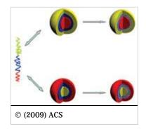
The co-polymer used by the researchers comprises three distinct polymer sections (see image). The middle section (blue) forms cross-link bonds with other co-polymer molecules, which prevent the micelles from falling apart. The outer sections (red and yellow) are two different polymers: one called PDEA, which becomes insoluble in
