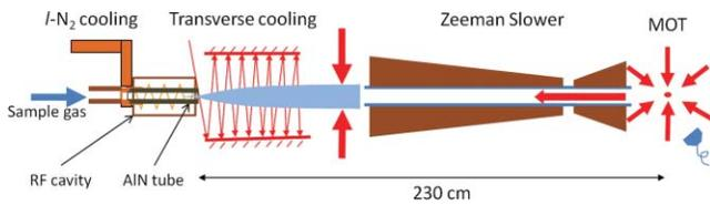
FIG. 1. (Color online) The schematic of the experimental setup.
