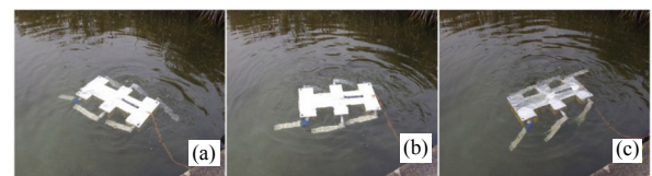
Fig. 13 Amphibious-I turning in water (anticlockwise).
