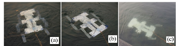
Fig. 12 Maneuvering in water. (a) Cruising; (b) backward swimming; (c) diving.
