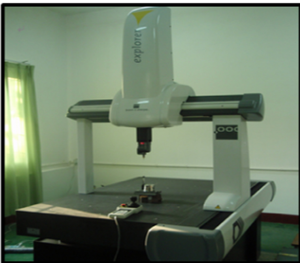
Fig. 3. Three-dimensional touch-probe measuring.
