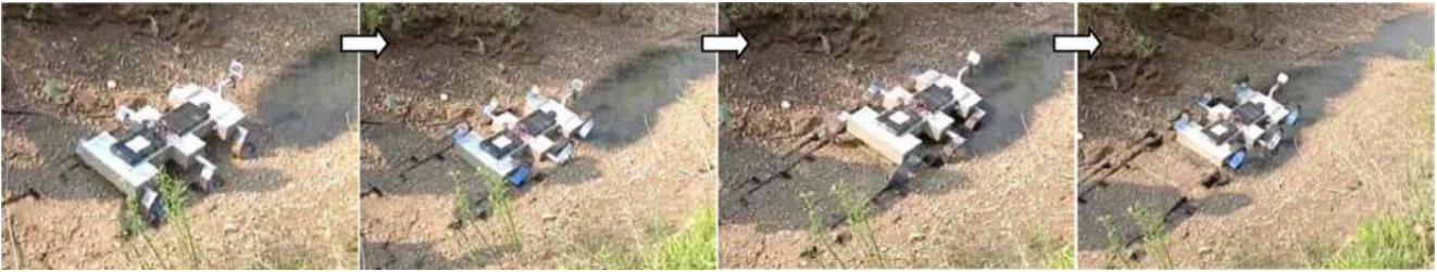
Figure 10 Snapshot sequence of the robot moving in field muddy terrain with hexapod gait
