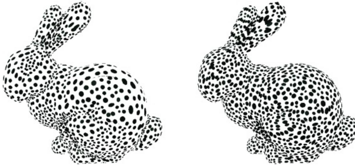
*Figure 4.28: Bunny model (see also Figure 4.30) decimated to similar number of splats by single-resolution OSS (left, 2,577) and progressive PSP (right, 2,591) algorithms. Although PSP and OSS have quite close errors (0.103% to 0.092%), being able to concentrate more splats on regions of high curvatures, OSS gives better splat shapes and distribution than PSP.*
