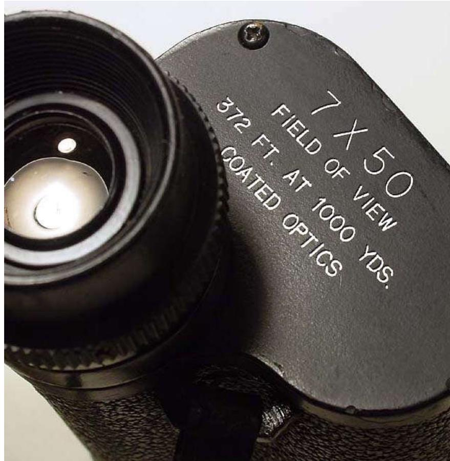
Parameters listed on the prism cover plate describing a 7 power magnification binocular with a 50 mm Objective diameter and a 372 feet Field of view at 1000 yards.
