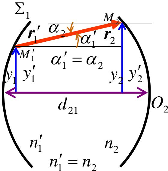
$$\begin{aligned}y_2 &\approx d_{21}\alpha'_1 + y'_1 \\n_2\alpha_2 &= n'_1\alpha'_1 + 0 \\y_2 &= (d_{21}/n'_1)n'_1\alpha'_1 + y'_1\end{aligned}$$
