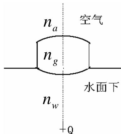
$$\begin{aligned} S &= \begin{pmatrix} 1 & -\Phi_2 \\ 0 & 1 \end{pmatrix} \begin{pmatrix} 1 & 0 \\ d/n_g & 1 \end{pmatrix} \begin{pmatrix} 1 & -\Phi_1 \\ 0 & 1 \end{pmatrix} \\ &= \begin{pmatrix} 1 & -16.67 \\ 0 & 1 \end{pmatrix} \begin{pmatrix} 1 & 0 \\ 0.02/1.5 & 1 \end{pmatrix} \begin{pmatrix} 1 & -5.67 \\ 0 & 1 \end{pmatrix} \\ &= \begin{pmatrix} 0.78 & -21.17 \\ 0.013 & 0.93 \end{pmatrix} \end{aligned}$$
