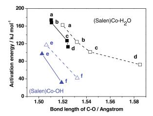
**Fig. 3.** The relationships between the activation energy and the bond length of PO's C–O bond to be broken at the initial states. The square (triangle) represents for the reaction via the Co-salen activated water (–OH), while the solid (open) symbol for the reaction via the primary (secondary) carbon. a–f represent for the different reaction pathways indicated in Fig. 2.
