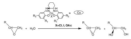
Fig. 1. Ring-opening hydrolysis reaction of the epoxides on the Co-salen catalysts.
