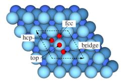
FIG. 1. (Color online) Top view of the high-symmetry adsorption sites (fcc, hcp, bridge, and top) on the Pt(111) surface. The  $(2\times2)$  unit cell is indicated by dashed lines. The Pt atoms and high-symmetry adsorption sites are indicated by large light blue balls and small red balls, respectively.
