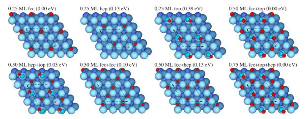
FIG. 2. (Color online) NO adsorption structures on Pt(111) in the  $(2 \times 2)$  unit cell (indicated by dashed lines) for different coverages and configurations. The Pt, N, and O atoms are indicated by large (light blue) balls, small blue, and red balls, respectively. The relative energy differences between different structures at given coverage are indicated in bracket.
