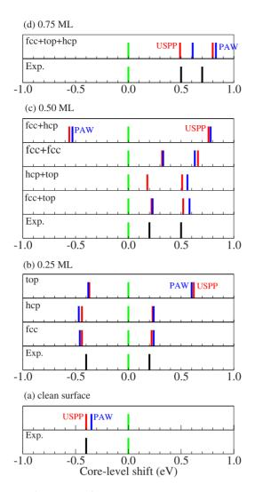
FIG. 7. (Color online) CLSs of the Pt 4f states in the topmost Pt(111) layer. (a) Clean surface. NO adsorption on Pt(111) for (b)  $\Theta_{\rm NO}$ =0.25, (c) 0.50 ML, and (d) 0.75 ML. The CLSs are given with respect to the bulk Pt atoms (center layer in the slab) and indicated by green lines. The USPP and PAW results are indicated in red and blue, respectively, while the experimental results (Ref. 9) are in black.
