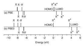
FIG. 3. (a) Electronic structure of NO in gas phase using DFT-PBE and (b) hybrid-DFT within the PBE0 functional. The highest occupied and lowest unoccupied molecular orbitals (HOMO, LUMO) are indicated along with the  $\pi$  and  $\sigma$  orbitals.
