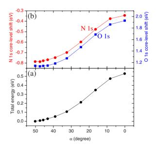
FIG. 8. (Color online) NO adsorption on Pt(111) in the (2  $\times$ 2)-2NO(fcc+top) structure. (a) Total energy and (b) core-level shift of the N and O 1s states as a function of the tilted angle ( $\alpha$  =0-50.2°) for NO in the top sites (see Fig. 4).  $\alpha$ =0 corresponds to optimized perpendicular top NO and  $\alpha$ =50.2° for optimized tilted configuration.
