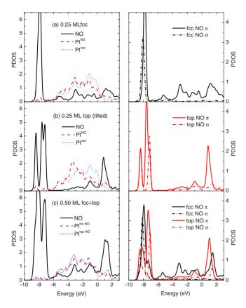
FIG. 6. (Color online) Projected density of states for NO/Pt(111) for (a) fcc and (b) top NO at 0.25 ML and (c) fcc+top (0.50 ML). In the left side, the total PDOS from adsorbed NO, bare surface Pt atoms (Pt<sup>vac</sup>), and surface Pt atoms coordinated with adsorbed NO (for instance Pt<sup>NO</sup>) are indicated. In the right side, the projected NO  $\sigma$  and  $\pi$  orbitals, defined in the main context, are plotted, respectively. The zero energy is the Fermi level.
