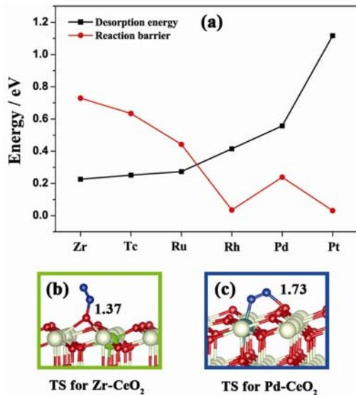
**Fig. 5.** (a) Correlations between calculated barriers (red) for N<sub>2</sub>O reduction and desorption energies (black) of N<sub>2</sub>O on TM<sub>1</sub>-Ov/CeO<sub>2</sub>(111); (b) The transition structure of linear N<sub>2</sub>O reduction on Zr<sub>1</sub>-Ov/CeO<sub>2</sub>(111); (c) The transition structure of bent N<sub>2</sub>O reduction on Pd<sub>1</sub>-Ov/CeO<sub>2</sub>(111).
