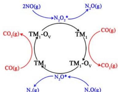
**Scheme 1.** Catalytic cycle for NO reduction by CO on TM<sub>1</sub>/CeO<sub>2</sub>(111) surface.
