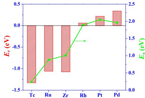
**Fig. 3.** Correlation between the reaction barrier and the reaction energy in the desorption of  $\text{N}_2\text{O}$  on  $\text{TM}_1/\text{CeO}_2(111)$  surfaces.
