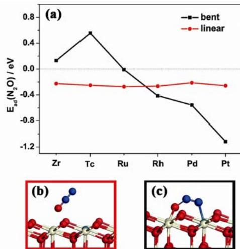
**Fig. 4.** (a) Adsorption energies of gaseous N<sub>2</sub>O on reduced TMs doped-CeO<sub>2</sub>(111) surfaces with bent (black) and linear (red) configurations, respectively; N<sub>2</sub>O adsorption on Pd<sub>1</sub>-Ov/CeO<sub>2</sub>(111) with linear (b) and bent (c) configurations, respectively.
