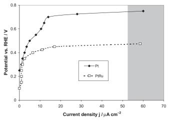
Fig. 12 Experimentally observed polarisation curve for CO (100%) oxidation at 62 °C on a platinum/ruthenium surface alloy electrode with the relative surface ratio of 50:50, reproduced from Ref. [12]. The shaded region shows the calculated range of equivalent current densities obtained from the experimental CO desorption rate for 100% CO, on varying the prefactor from  $10^{13}$  to  $10^{17}$ , and extrapolated to 62 °C.
