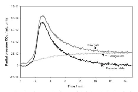
Fig. 3 The evolution of  $CO_2$  arising from the titration of adsorbed CO with 1 bar of  $O_2$ . The subtraction of the background obtained due to reaction of oxygen in the mass spectrometer is also shown.
