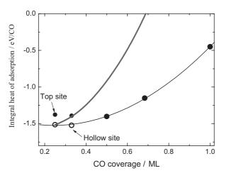
Fig. 7 The integral heats of adsorption for CO on Pt(111) at different coverages calculated using DFT. The lower thin line is the second order polynomial fit to the most stable adsorption configuration whilst the upper thick line gives the differential heat of adsorption.
