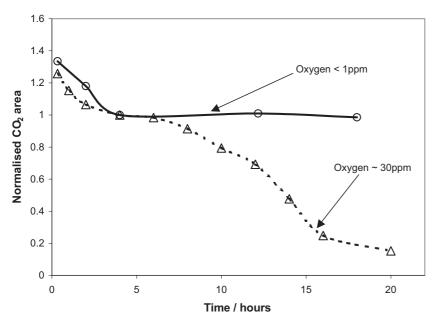
Fig. 4 Plot of normalised CO<sub>2</sub> peak area against time of exposure. CO is dosed at 1 bar, then replaced by a flow of argon. After a given exposure time the remaining CO is titrated with  $O_2$  to produce CO<sub>2</sub>. Data is shown for an oxygen-free and oxygen contaminated system.
