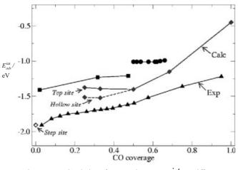
Fig. 2 The integrated enthalpies for CO adsorption ( $E_{ads}^{int}$ ) at different coverages. The DFT results (diamonds) are compared to three different sets of experimental results (triangles, circles and squares) taken from [33], where differential enthalpies have been changed to integrated enthalpies for comparison with the calculated results. The enthalpy for CO adsorbed at a step site (open diamond) is taken from [41].
