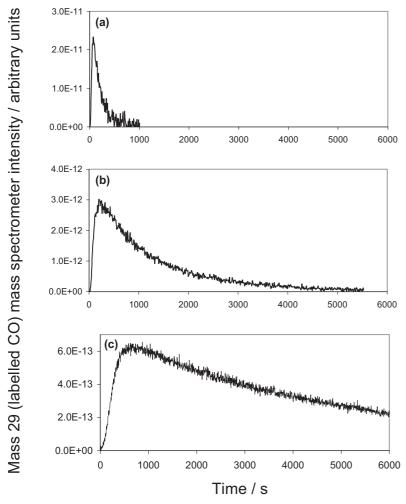
Fig. 5 Plots showing C<sup>13</sup>O desorption in flows of: (a) 1 bar CO, (b) 1000 ppm CO in argon and (c) 100 ppm CO in argon from the platinum electrocatalyst.
