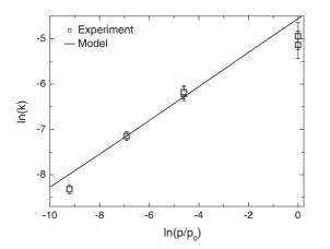
Fig. 11 Plot of the rate of  $C^{13}O$  desorption versus the pressure of  $C^{12}O$  above the surface. Squares represent experimental data whilst the solid line is from the simple model described in the text.
