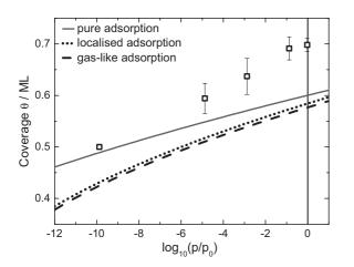
Fig. 10 The experimental data shows the CO coverage versus the CO pressure as measured with the HP STM. Also shown is the calculated equilibrium coverage of CO on the Pt(111) surface at room temperature (see text). The solid line represents the adsorption model not including any effects related to the statistics of CO adsorption on the surface. The dotted line is for the lattice gas model, and the dashed line represents a model of the mobile CO at the surface.
