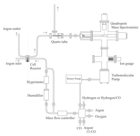
Fig. 1 Apparatus used for flow data measurement.
