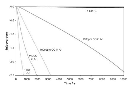
Fig. 6 Plot of ln of the normalised coverage versus time for a preadsorbed overlayer of  $C^{13}O$  under flows of various gases and gas mixtures.
