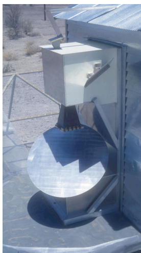
Figure 41: A refined experiment to look for anisotropy in the CMBR. Note the inverted horn and the use of ground screens to minimize stray radiation from the ground.
