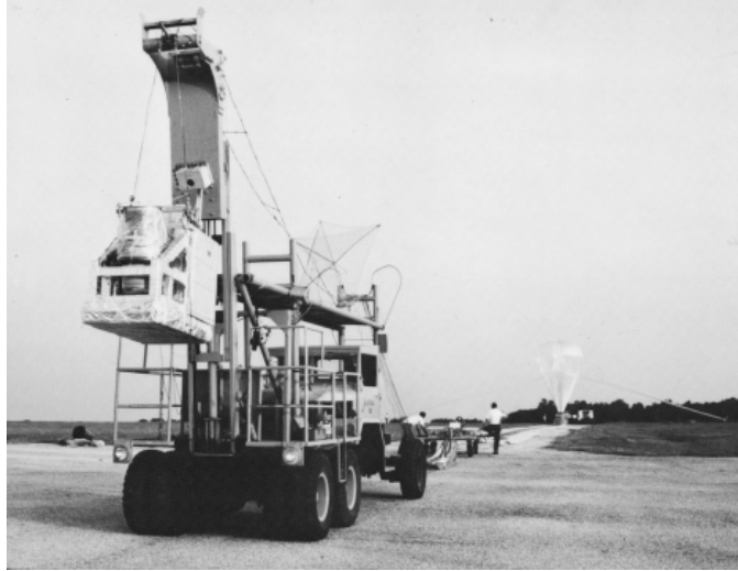
Figure 34: The launch layout for the first flight of the new payload. The package has been lifted by the launch vehicle ASCEND II. The payout reel with the 700 meters of line is on the cart between the launch vehicle and the balloon. At the time when the picture was taken the top of the balloon was being filled with helium. The lower part of the balloon is lying on a tarpaulin between the cart and the clamp that is holding the balloon down. Although they are not visible, there are separate parachutes in the flight train for the reel and the payload. Once the balloon is released the launch crew member with his foot on the cart will follow the path of the balloon as it lifts the reel off the cart. ASCEND II will chase the balloon around the field until it is a little down wind of the vehicle and then release the payload. If the launch master has been successful, the payload will go forward and upward rather than backwards and hit the vehicle. The launch ballet and the balloon dynamics are lovely to watch and much quieter than a spacecraft launch.
