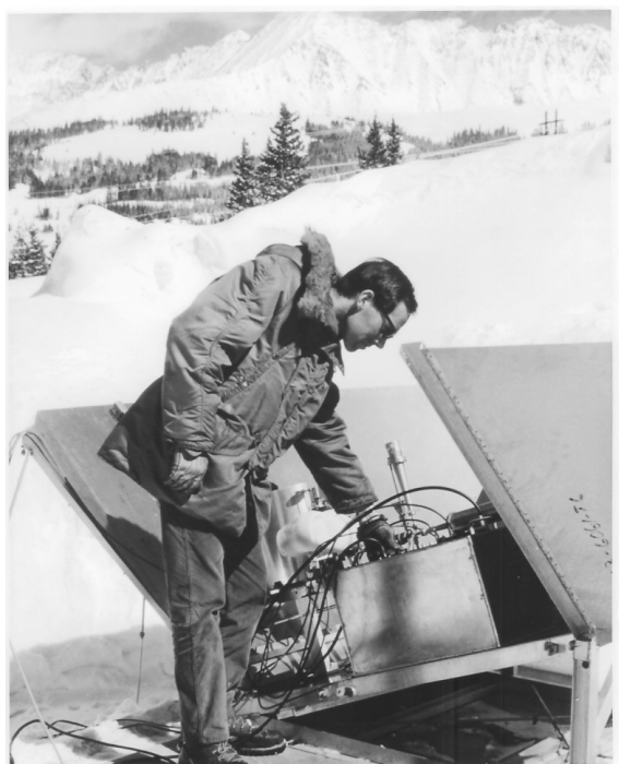
Figure 27: Robert Stokes with a 3.3-mm Radiometer — Colorado 1968.
