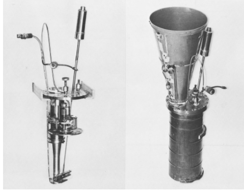
Figure 31: Left: photograph of the radiometer showing the filter transport and chopper; right: the sealed copper can with the radiometer installed.
