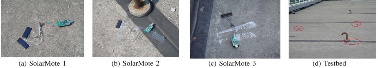
Fig. 6. TelosB nodes with solar charging cells.
