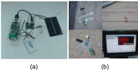
Fig. 1. (a) TelosB nodes with solar charging cells; (b) Our TestBed.
