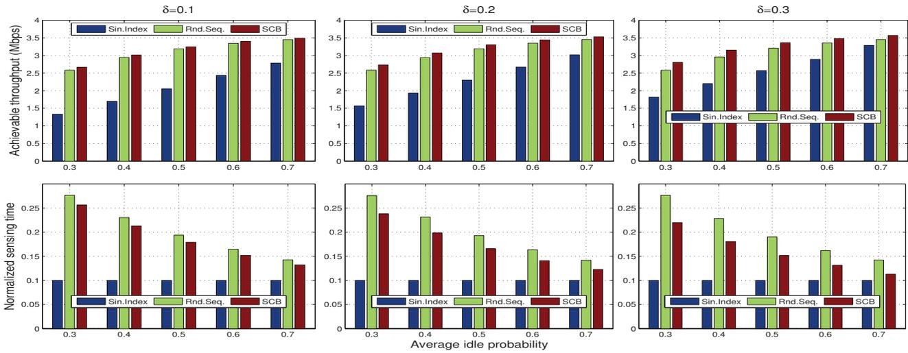
Fig. 10. Achievable throughput &amp; normalized sensing cost vs. idle probability distribution
