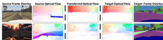
Figure 6: Examples of motion translation results in video-to-labels. From left to right: Source frame overlay, optical flow in source, transferred optical flow via motion translator, ground truth optical flow in target, and ground truth target frame overlay.
