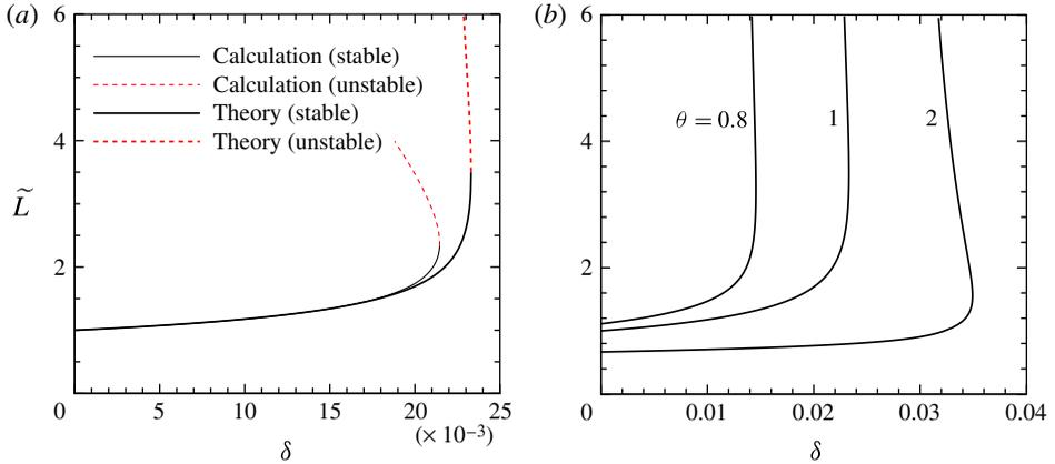
FIGURE 4. (a) Variation of  $\tilde{L}$  as a function of  $\delta$  for the symmetric case. The theoretical solutions (thick lines) are given by (4.15). Numerical results (thin lines), obtained by directly integrating the governing equation (4.1) with  $\theta_l = \theta_r = \pi/6$ , are also plotted for comparison. (b) Effect of the contact angle ratio  $\theta$ . The dimensionless slip length is  $\lambda = 10^{-6}$ .
