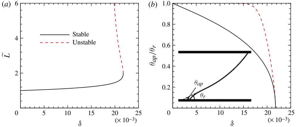
FIGURE 2. Variation of (a) the rescaled contact-line distance  $\tilde{L} = \theta_r L$  and (b) the apparent contact angle  $\theta_{ap}/\theta_r$  as functions of  $\delta$  for  $\lambda = 10^{-7}$  and  $\theta = 1$ . The definition of  $\theta_{ap}$  is schematically shown in the inset. The stationary solutions only exist for  $\delta \leq \delta_c = 0.0218$ .
