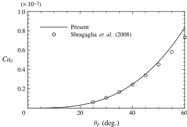
FIGURE 3. Comparison of the critical capillary number  $Ca_c$  for  $\lambda = 10^{-7}$  and  $\theta = 1$  with the numerical results of Sbragaglia *et al.* (2008).
