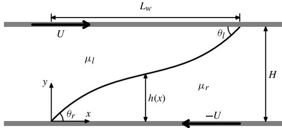
FIGURE 1. Schematic of the shear flow driven by two parallel walls moving in opposite directions with velocity  $\pm U$ . The line  $h(x)$  represents the fluid–fluid interface.
