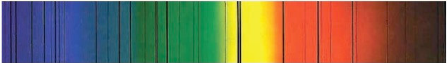
Figure 2.4 The solar spectrum showing the Fraunhofer lines. The peak intensity is in the yellow part of the spectrum close to the strong pair of sodium D lines in the centre of the spectrum.
