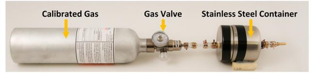
**Figure 9: Our ADC to concentration mapping process involves industrial calibrated gas, a gas valve with flow rate control, a stainless steel container and necessary anti-corrosive tubes and connectors.**
