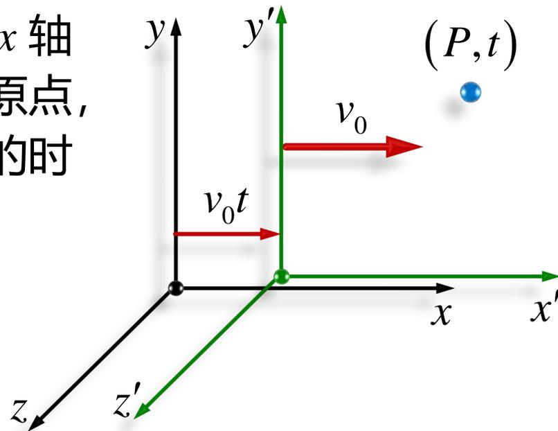
$$\begin{pmatrix} ct' \\ x' \\ y' \\ z' \end{pmatrix} = \begin{pmatrix} \gamma_0 & -\beta_0 \gamma_0 & 0 & 0 \\ -\beta_0 \gamma_0 & \gamma_0 & 0 & 0 \\ 0 & 0 & 1 & 0 \\ 0 & 0 & 0 & 1 \end{pmatrix} \begin{pmatrix} ct \\ x \\ y \\ z \end{pmatrix}$$
