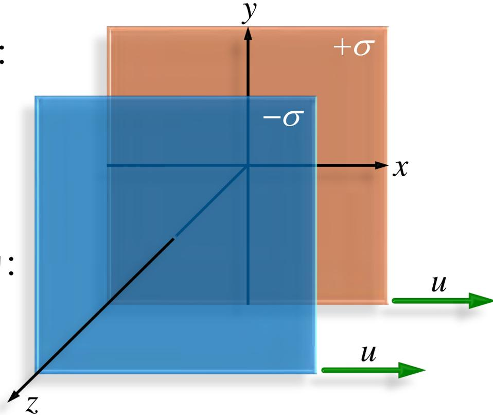
$$\longrightarrow E'_z = \gamma_0 \left( E_z + v_0 B_y \right), \quad B'_z = \gamma_0 \left( B_y + \frac{v_0}{c^2} E_z \right)$$
