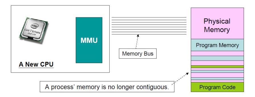
Step 1. When CPU wants to fetch an instruction, the virtual address is sent to MMU and is translated into a physical address.
