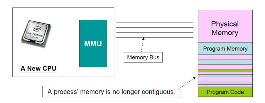
Step 1. When CPU wants to fetch an instruction, the <u>virtual address</u> is sent to MMU and is translated into a <u>physical address</u>.
