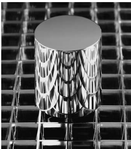
Figure 1. The U.S. national prototype kilogram, K_{20} .
