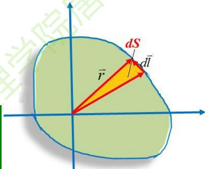
$$\vec{M} = \oint_L \vec{r} \times (I d\vec{r} \times \vec{B}) = I \left( \frac{1}{2} \oint_L \vec{r} \times d\vec{r} \right) \times \vec{B} = \vec{\mu} \times \vec{B}$$
