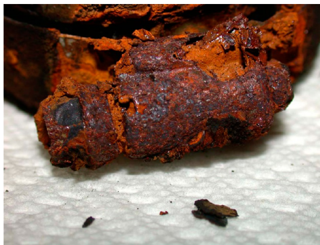
Figure 1. Photograph showing the corrosion or rusting of a piece of steel. Reproduced with permission from ref 83. Copyright 1996 Bushman & Associates.
