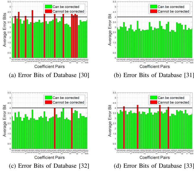
Fig. 12: The average error bit corresponding to different coefficient pairs.
