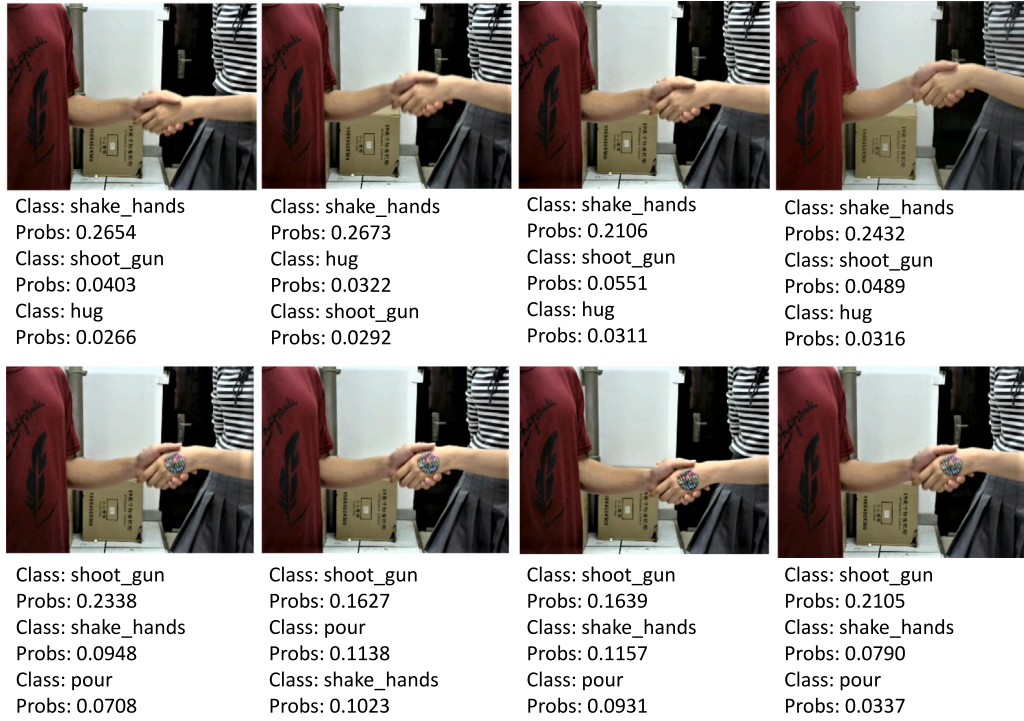
Fig. 1. This figure shows the physical attack results of real-time action recognition models. The first line contains the adversarial videos, and the second line includes the original videos after adding an adversarial patch to the palm. The ‘shake-hands’ action can be mistaken for ‘shoot-gun’. The radius set in this experiment is 50 pixels. At the bottom of each image is the label of the current frame.
