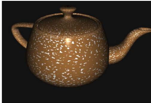
We use the noise texture to vary the color of the object, with a sharp transition between the base color and the paint color. We'll use either the base color or paint color as the diffuse reflectivity of the shading model. If the noise value is above a certain threshold, we'll use the paint color; otherwise, we'll use the base color of the object.
