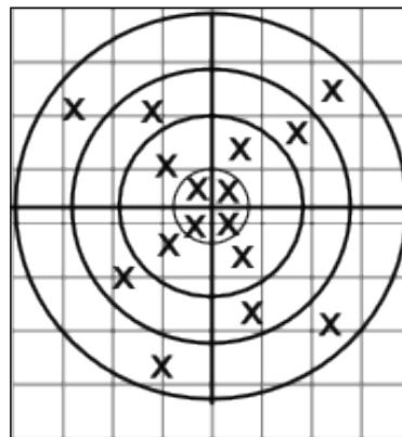
Additionally, we vary the sample locations through a set of precomputed sample patterns. We compute random sample offsets and store them in a texture prior to rendering. Then, in the fragment shader, the samples are determined by first accessing the offset texture to grab a set of offsets and use them to vary the fragment's position in the shadow map. The results are then averaged together in a similar manner to the basic PCF algorithm.
