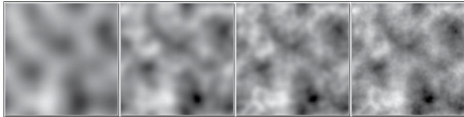
In this recipe, we'll store all four values in a single 2D texture. We'll store Perlin noise with one octave in the first component (red channel), two octaves in the green channel, three octaves in the blue, and four octaves in the alpha channel.
