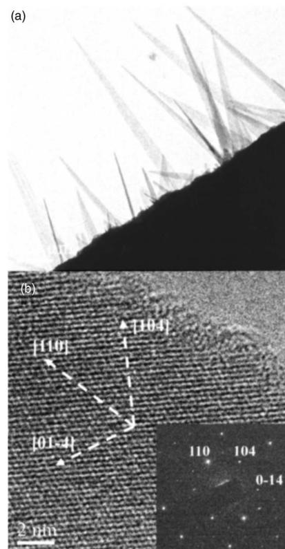
FIG. 2. (a) Typical TEM image of  $\alpha$ -Fe<sub>2</sub>O<sub>3</sub> nanoflakes on an AFM tip. (b) HRTEM image from a long  $\alpha$ -Fe<sub>2</sub>O<sub>3</sub> nanoflake. From it, the lattice fringe is measured as about 2.71 Å, consistent with the interplanar spacings of both (104) and (01 $\bar{4}$ ) in  $\alpha$ -Fe<sub>2</sub>O<sub>3</sub>. The inset shows corresponding SAED pattern, which can be indexed with crystal zone of  $[\bar{4}41]$ .
