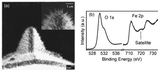
FIG. 1. (a) Typical SEM image of  $\alpha$ -Fe<sub>2</sub>O<sub>3</sub> nanoflakes on an AFM tip. Inset shows a high magnification SEM image of the tip apex. (b) XPS spectra of O 1s and Fe 2p from as-grown samples.
