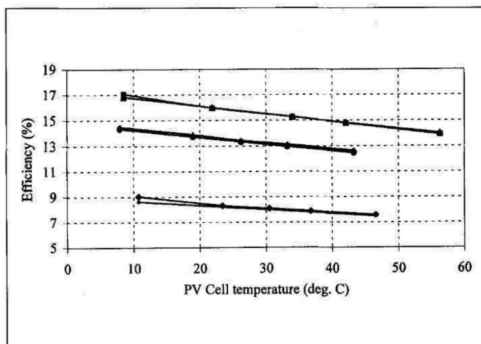
Figure 8 – Comparisons between Simulation and Test Results for the Three PV Modules
