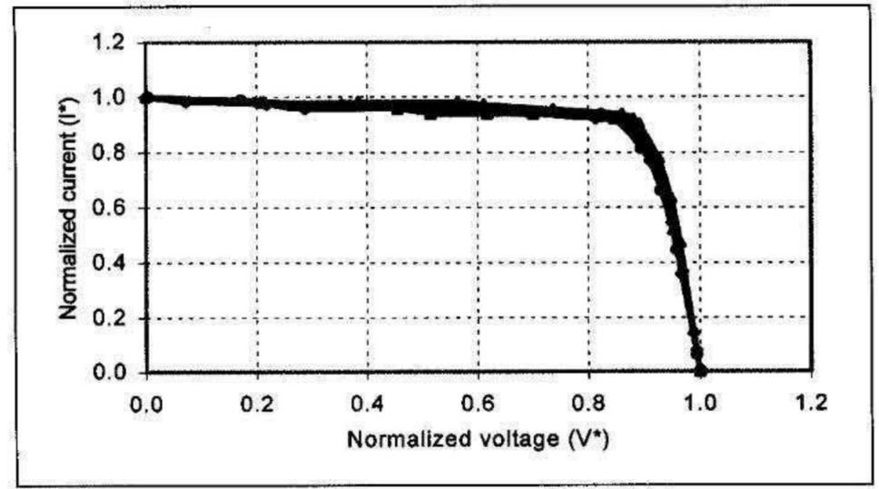
Figure 3 – Normalized Current and Voltage for Different Cell Temperatures for Module A
