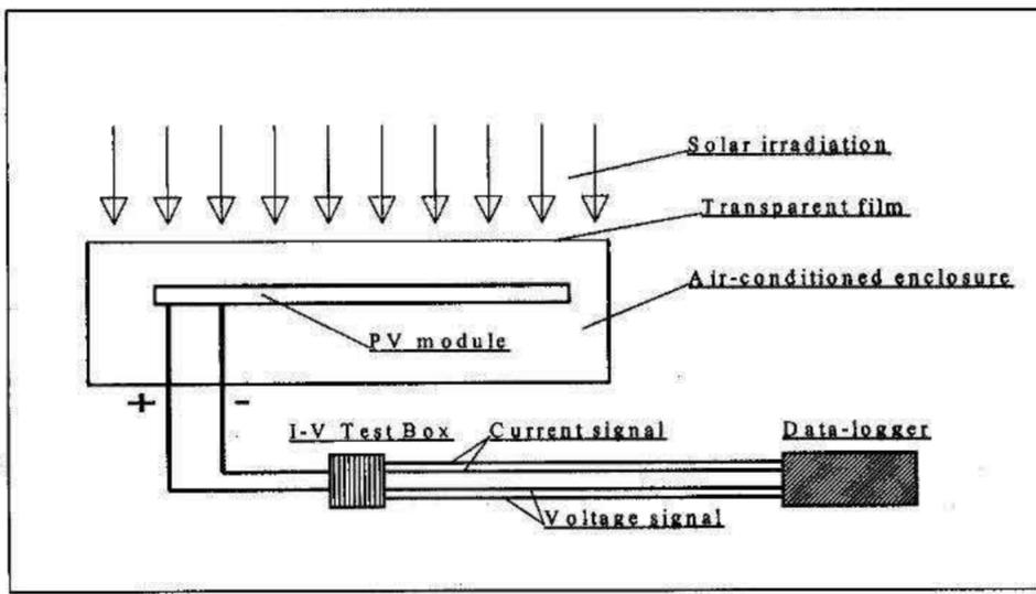
Figure 1 – I-V Characteristics Test Set-Up
