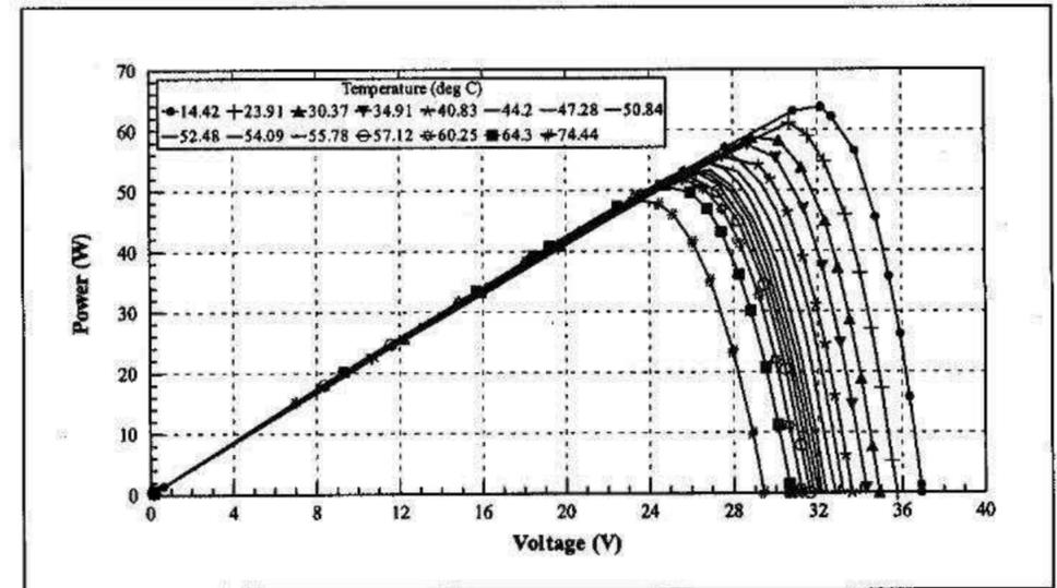
Figure 4 – Power Output from PV Module A
