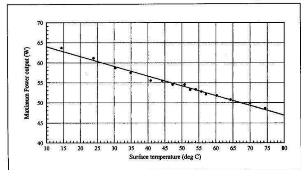
Figure 5 – Maximum Power Output vs PV Surface Temperature for PV Module A
