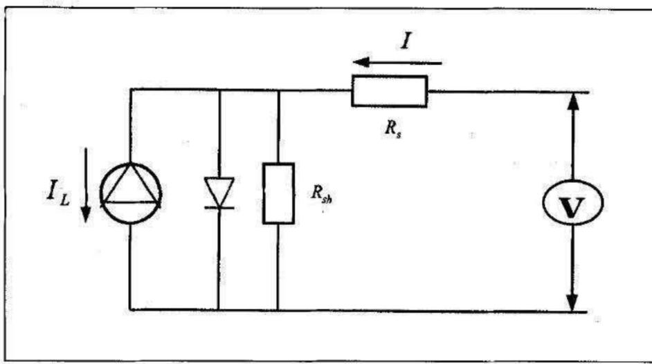
Figure 6 – Circuit Representation of a Solar Cell System
