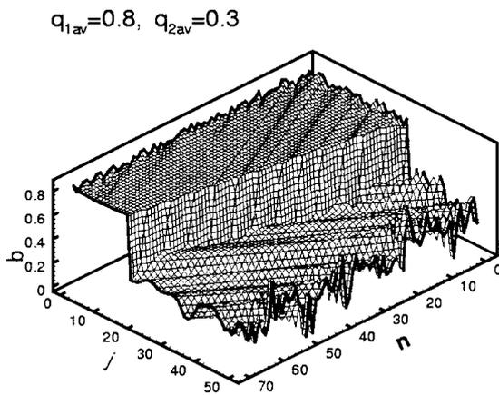
**Fig. 5.** 3D presentation of traffic flow rate, where  $j=x/\Delta x$ ,  $n=t/\Delta t$
