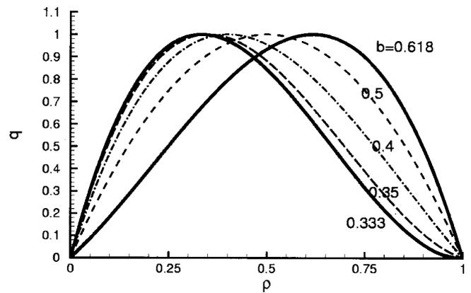
**Fig. 1.** Traffic flow-density diagram for several values of parameter  $b$
