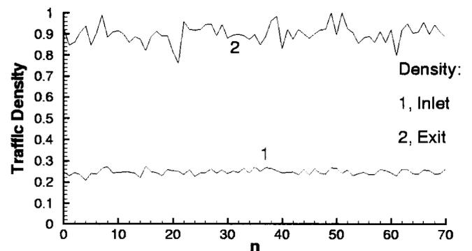
Fig. 2. Inlet and exit traffic densities predicted by computer-based random generator, which was constructed in terms of Erlang process of order 250
