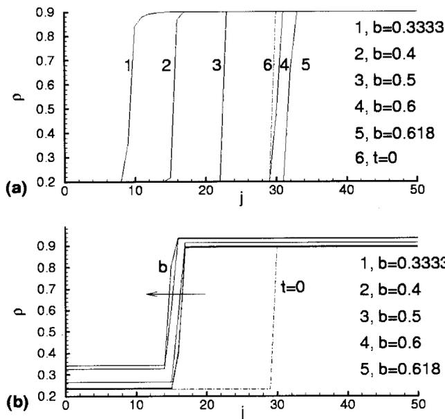
**Fig. 3.** Traffic shock wave shapes and locations at time  $n = t/\Delta t = 70$  for several values of single parameter, where: (a) for  $\rho_1 = 0.2$ ,  $\rho_2 = 0.8$ ; (b) for  $q_1 = 0.8$ ,  $q_2 = 0.3$ ; and  $j = x/\Delta x$
