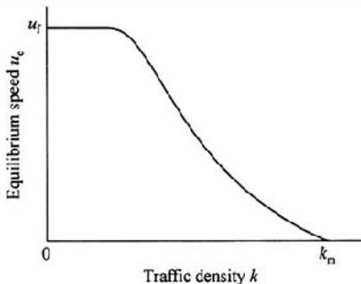
Fig. 1. A typical equilibrium speed-density curve, where  $u_f$  is free flow speed,  $k_m$  is jam density.
