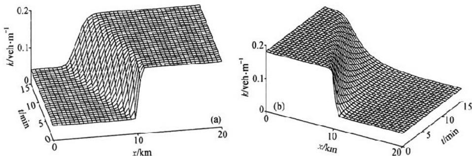
Fig. 2. The spatiotemporal evolution of density under different Riemann initial conditions. (a) For condition ( i ); (b) for condition ( ii ).
