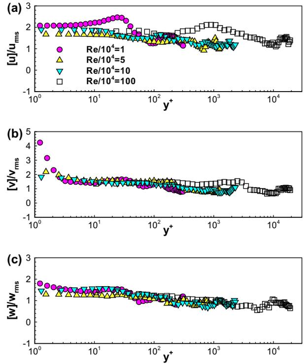
**Fig. 3.** The velocity variation bands along the wall-bisector plotted as functions of the wall coordinate at various Reynolds numbers. (a)  $[u]/u_{rms}$ ; (b)  $[v]/v_{rms}$ ; and (c)  $[w]/w_{rms}$ .
