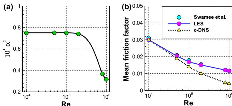
**Fig. 1.** The sub-grid viscosity at  $y^+ \rightarrow \infty$  (a) and the friction factor (b) plotted as functions of bulk Reynolds number. Note that the value of  $\alpha^2$  is determined by calibrating the friction factor with the explicit expression of Swamee and Jain [59]:  $f = 0.25 / \{\log[k_s / (3.7H) + 5.74 / Re^{0.9}]\}^2$ , which is introduced in the book of Roberson and Crowe [60], where the equivalent sand roughness  $k_s$  was set as zero in the calibration.
