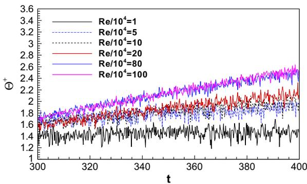
Fig. 8. The dependence of the evolution of normalized temperature at the origin point  $(0, 0, 0)$  on the Reynolds number, in which the data acquisition interval is set as  $50\Delta t$ .
