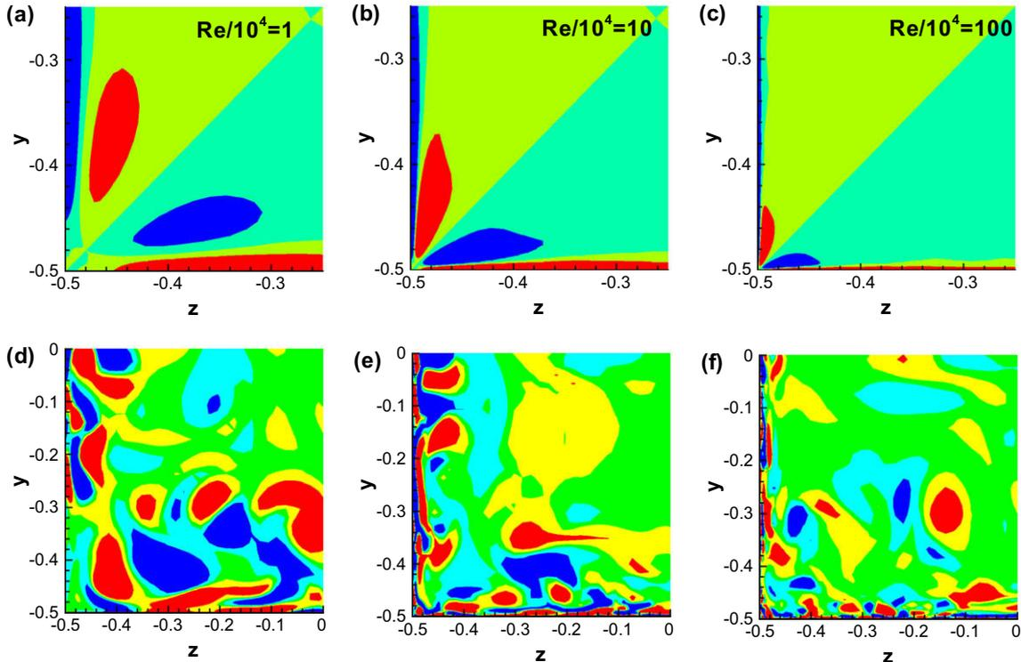
Fig. 6. The comparison of the quadrant-averaged mean secondary flows (a–c) with the instantaneous secondary flows (d–f) in the third quadrant at the time of 360 at the Reynolds number of  $10^4$ ,  $10^5$  and  $10^6$ , respectively. Note that the contours in (a–c) are labeled by vorticity values of  $-0.5$ ,  $0$ , and  $0.5$ , while the contours in (d–f) are labeled by  $-2$ ,  $-0.5$ ,  $0.5$ , and  $2$ .
