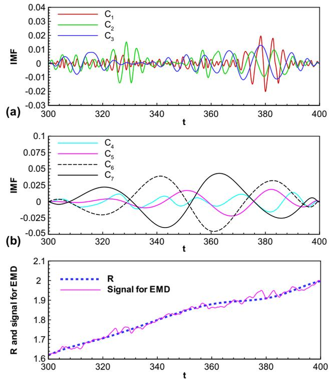
Fig. 9. The intrinsic mode functions (IMF) of  $x$ -averaged cross-sectional origin temperature in the unit of  $13T_z$  (a and b), and the residual  $R$  and signal for the empirical mode decomposition (EMD) (c) at the Reynolds number of  $10^5$ .
