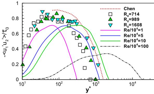
Fig. 5. The comparison of Reynolds shear stress along the wall-bisector with experiments and theoretical analysis. The  $R_0$  in the work of Chen et al. [19] is around 1600. While the angular bracket is used to denote the time and  $x$ -averaging.
