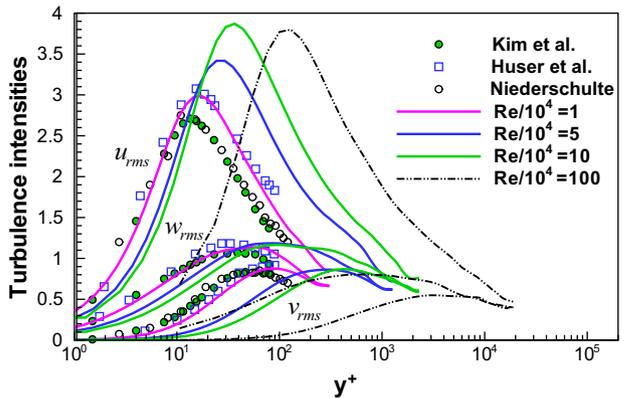
**Fig. 4.** The comparison of turbulence intensity along the wall-bisector with existing data. Note that the friction Reynolds number is 180 (based on the channel half-width and wall shear velocity) in the fully spectral DNS of the plane channel flow done by Kim et al. [30], and in the experiment with laser-Doppler techniques by Niederschulte et al. [37]. In the DNS of Huser and Biringen [24]  $Re_\tau = 600$ .
