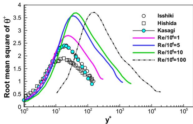
**Fig. 10.** The comparison of the rms curve of temperature along the wall-bisector with existing results. Note that the friction Reynolds number is 150 (based on the channel half-width and wall shear velocity) in the fully spectral DNS of the plane channel flow done by Kasagi et al. [32], and the data labeled by 'Isshiki' abstracted indirectly from [32]. The friction Reynolds number in the work of Hishida et al. [62] is 879.
