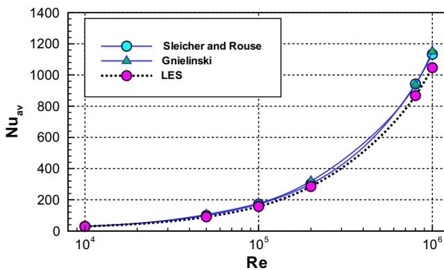
**Fig. 11.** The comparison of overall mean Nusselt number with experiments. Note that the correlation of Gnielinski was indirectly abstracted from Ref. [65].
