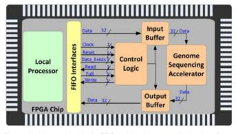
Fig. 6. Architecture in single FPGA chip, the cmmunication interfaces between processor and accelerator is based on FIFO interface.
